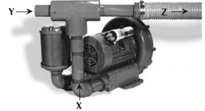
(X) Motive air; (Y) Product pick-up with vacuum flow; (Z) Air exhaust from "X" and material from "Y"
